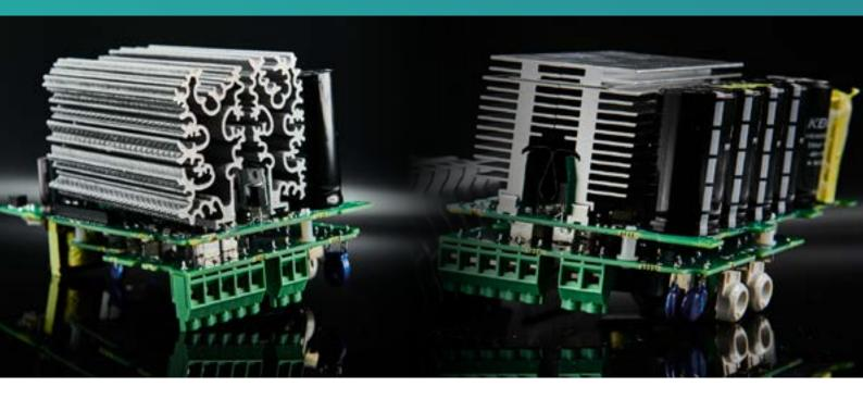
Utilising thermal-fluid topology optimisation and additive manufacturing to address the issues of performance, miniaturisation, and weight in traditional heat sinks
