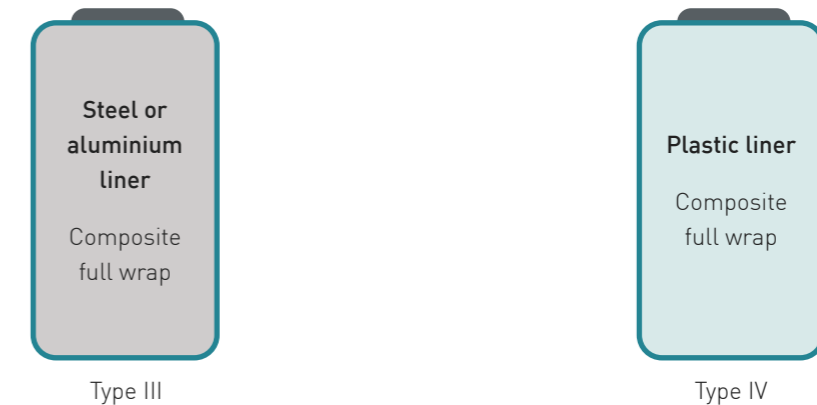
Figure 13: Lightweight Composite Hydrogen Storage Container Types [3].
