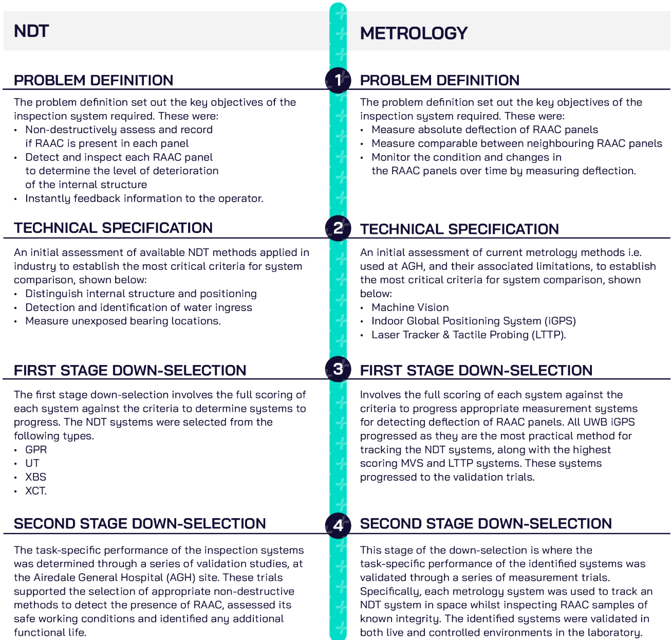
Figure 33: MTC's standard down-selection process to determine the most appropriate inspection systems for RAAC
