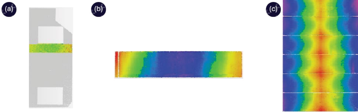
Figure 49: (a) Panel measured by BLK2GO, (b) panel measured by ATS 600, (c) deflection map of ceiling.
