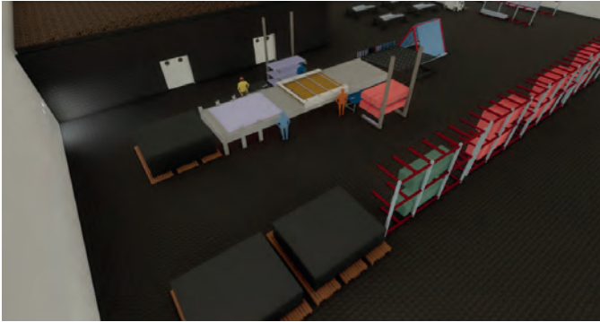
Figure 12. View of virtual partition wall assembly line
